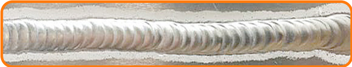
TH : 3mm Amp: 120A Wave : Triangular
